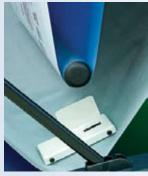
Contact-free sensor. The sensor positioned below the loop works without direct contact.
